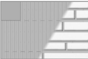
The staggered saw-cuts form an optical straight line, enabling the lengthwise connected decking boards to be fixed on a double eco-beam.
