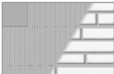
The staggered saw-cuts form an optical straight line, enabling the lengthwise connected decking boards to be fixed on a double eco-beam.
